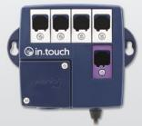
The in.touch module has a built-in WiFi transceiver that allows it to communicate with your devices.
