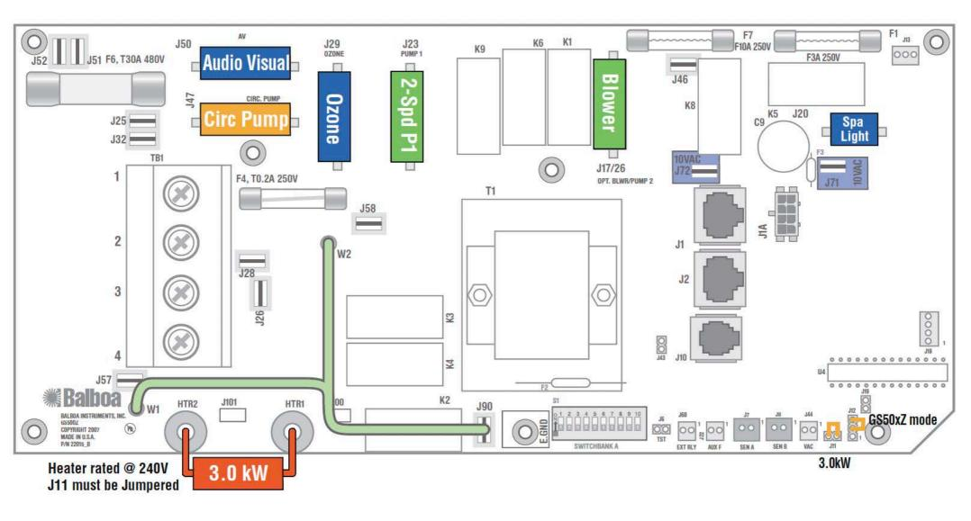
WARNING: Main Power to system should be turned OFF BEFORE adjusting DIP switches.
