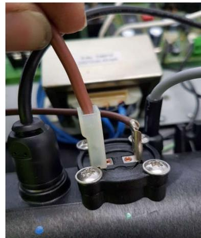
16. Connect the brown wire from the element wiring to the POH1 connector on the circuit board.
