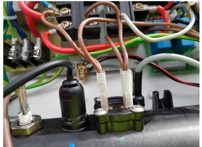
14. Gently lay the element into the unit, slipping the element tube feet under the screws in the bottom. Tighten the screws to secure the element.
