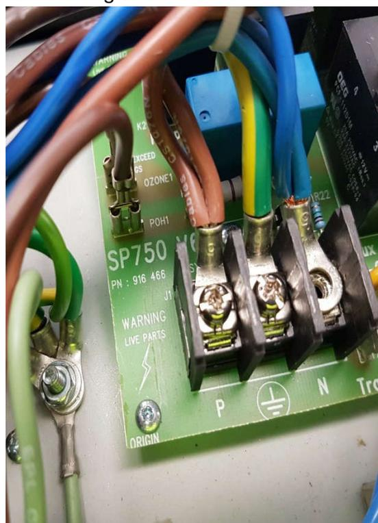
17. Connect new element blue neutral wire to screw terminal block and secure it with the screw.
