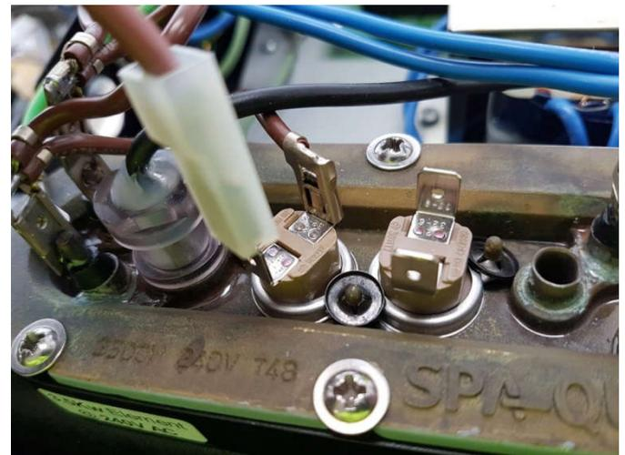
7. Remove the element earth screw and remove the green/yellow earth wire.
