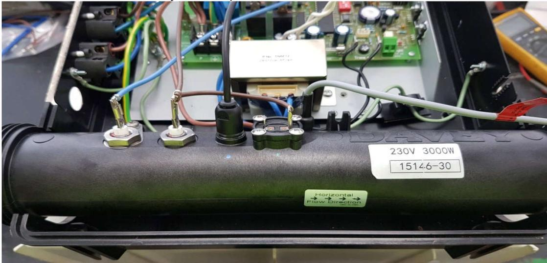
12. Unwind the white wires and remove the white wire that is connected to the KL2 terminal. The removed white wire is no longer required and can be discarded.
